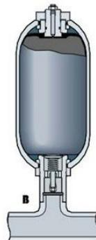
B- An inert gas (nitrogen) is introduced into the bladder through a special valve with pressure  $P_0$ . The bladder expands, filling the entire volume  $V_0$  of the accumulator shell.
