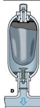
D- When the liquid pressure rises to  $P_2$ , the volume of gas reduces to  $V_2$  with an attendant rise in pressure, thus balancing the liquid pressure. This means that the accumulator has been pressurised  $\Delta V = V_1 - V_2$  and a potential energy has been created to be utilised as desired.
