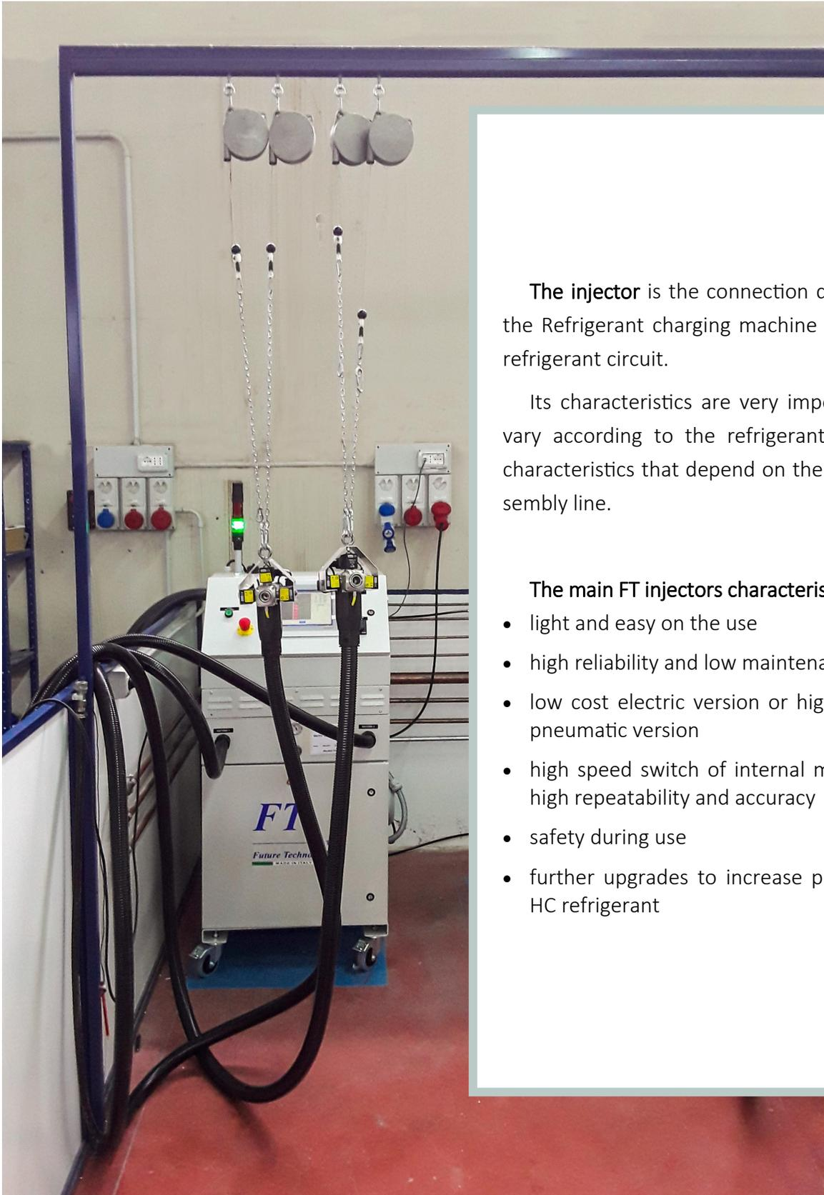
The **injector** is the connection device between the Refrigerant charging machine and the cooler refrigerant circuit.
