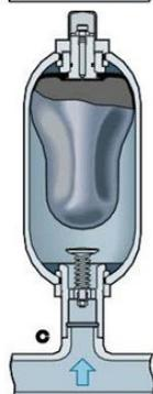
C- When circuit pressure  $P_1$  is higher than the gas pre-charge pressure  $P_0$ , the liquid valve opens, and the bladder is compressed reducing the gas volume to  $V_1$ .
