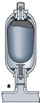
A- A flexible separator bladder is fitted into a pressure vessel (accumulator shell).
