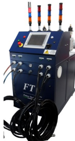
iAmiata for pressure stress test
