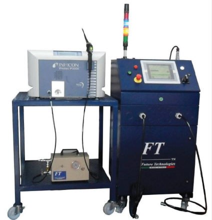
iAmiata connected to leak detector
